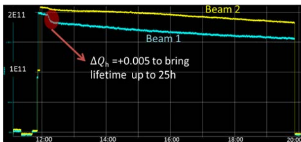
Figure 2: Total beam intensity evolution during Fill 1069. Beam 1 is shown in blue while Beam 2 is shown in yellow.
